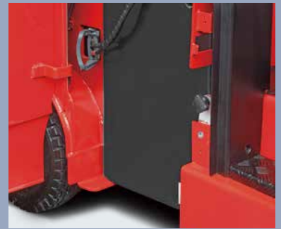
The battery can be removed from truck side, so it is very convenient for battery maintenance
