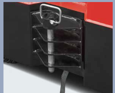
Upon special design, the traction device can prevent the towing pin coming off during traveling
